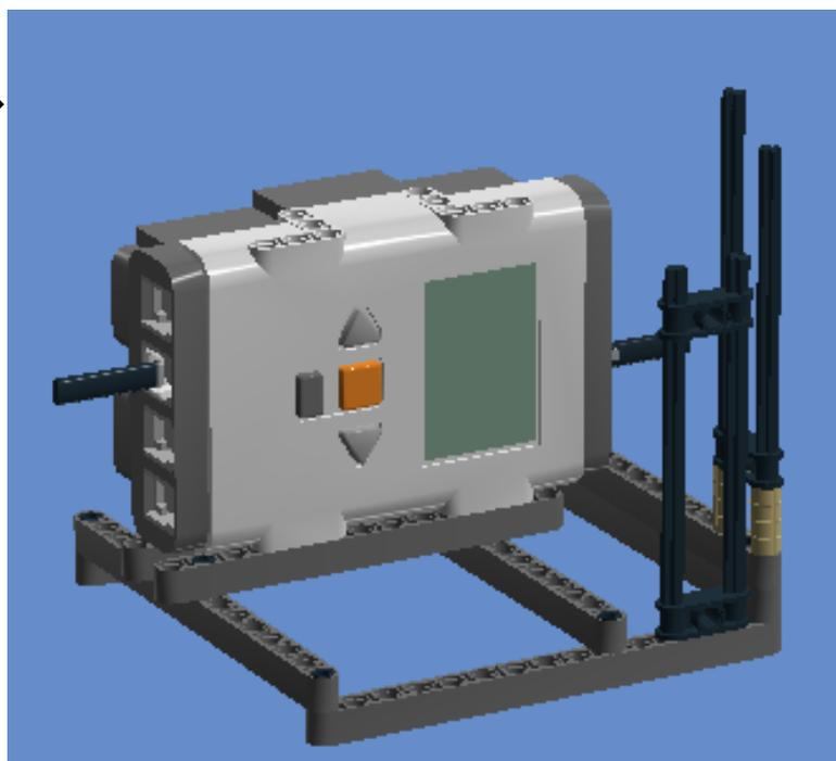
**11° Passo:** Technic 5m beam, Technic 7m beam, Connector Peg w. Friction e Connector peg w. friction 3m.
