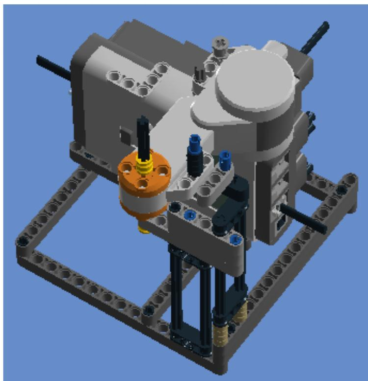
**20° Passo:** 1/2 Bush, Technic 5m Beam, Technic 3m Beam e Gear Wheel 40T.
