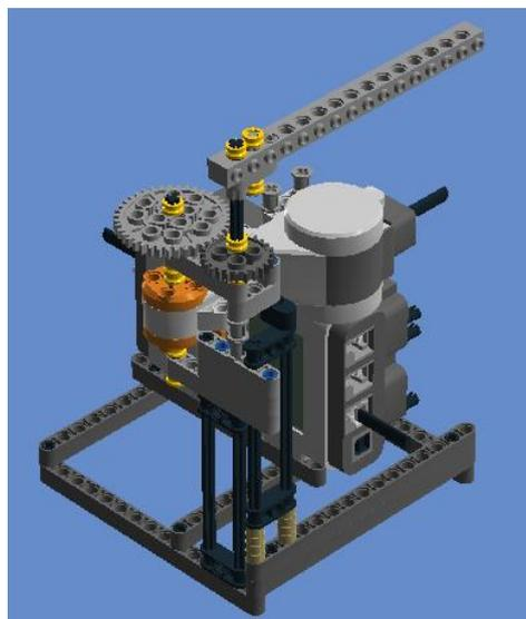
**24° Passo:** Technic 5m Beam, Technic 7m Beam, Connector peg w. friction 3m, Connector Peg w. Friction e Angular beam 90degr. w.4 snaps.
