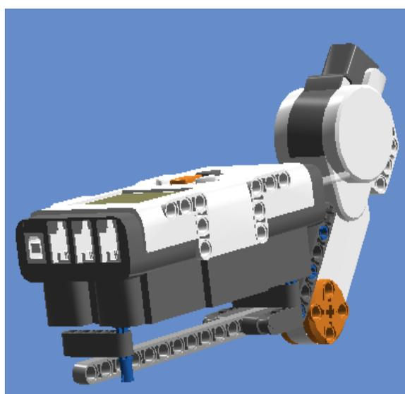
**7° Passo:** Connector peg w. friction 3m, Cross block 90° e Technic ang. beam 4X2 90 deg.
