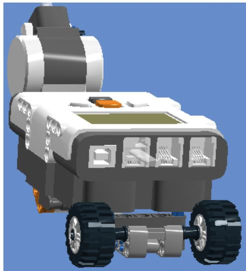
**11º Passo:** Connector peg/cross axle, Connector peg e Technic angular beam 4X6 –
